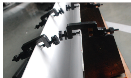
图7 C形定力夹紧装置示意图 Fig.7 Schematic diagram of C-shaped clamping device
