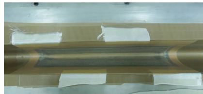
图16 铺层交叉间隔固持示意图 Fig.16 Schematic diagram of cross interval grasped layer
